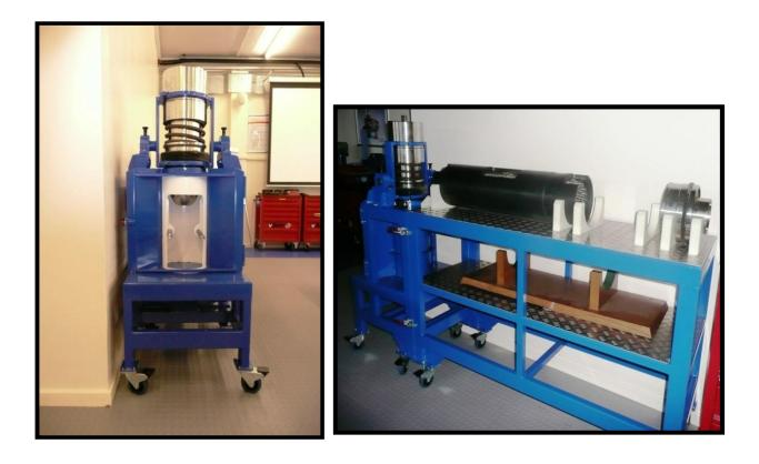
This product is designed to assist in training staff in the correct method of swaging the end fittings to the tie bar.
